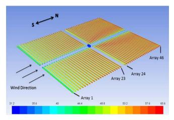
Fig. 10. Module temperatures from 3-D simulations of air flows and thermal exchange during a sunny day
