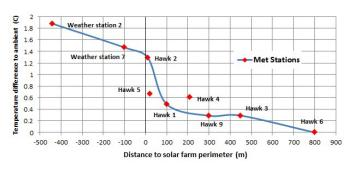
Fig. 8. Air temperature difference as a function of distance from the perimeter of the solar farm. Negative distances indicate locations within the solar farm.
