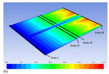
Fig. 11 Air temperatures from 3-D simulations during a sunny day. a) Air temperatures at a height of 1.5 m; b) air temperatures at a height of 2.5 m.
